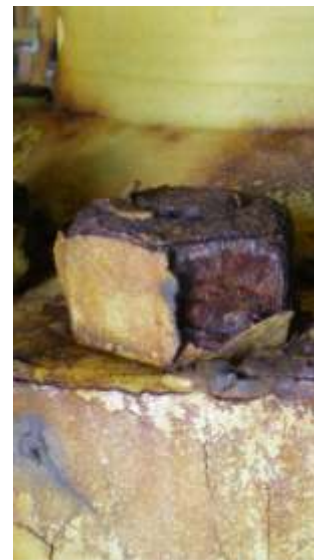
Left and below: platform viewed from the sea; well head showing heavy corrosion with closer details of corrosion effects on flanges and bolts.
