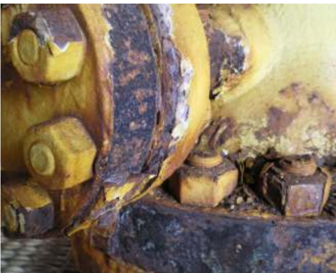
Below and right: removal of corrosion shows condition of substrate. The depth of corrosion is clearly visible as corrosion scale is removed. It was not possible to completely remove corrosion between flange faces.
