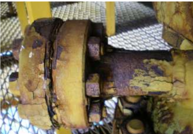
Below and right: removal of corrosion shows condition of substrate. The depth of corrosion is clearly visible as corrosion scale is removed. It was not possible to completely remove corrosion between flange faces.
