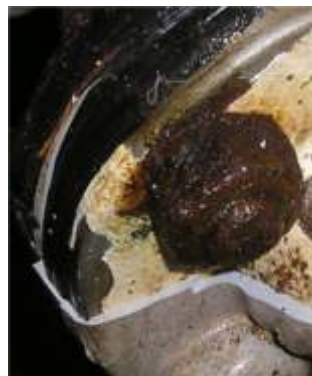
Above: after two years, an application on a flange with severely corroded bolts is cut away for inspection. No further corrosion has taken place and inhibiting oil can be seen on the fastening and in the removed Enviropeel coating.
