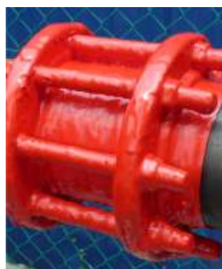
Above: after two years, an application on a flange with severely corroded bolts is cut away for inspection. No further corrosion has taken place and inhibiting oil can be seen on the fastening and in the removed Enviropeel coating.
