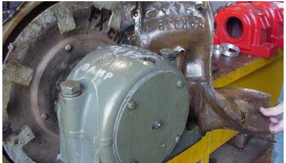
Below: With the Enviropeel removed from a pulley housing after use, it is clear how good the performance of the Enviropeel is. The roller in the background shows clear evidence of corrosion whereas the protected pulley is as good as new.
