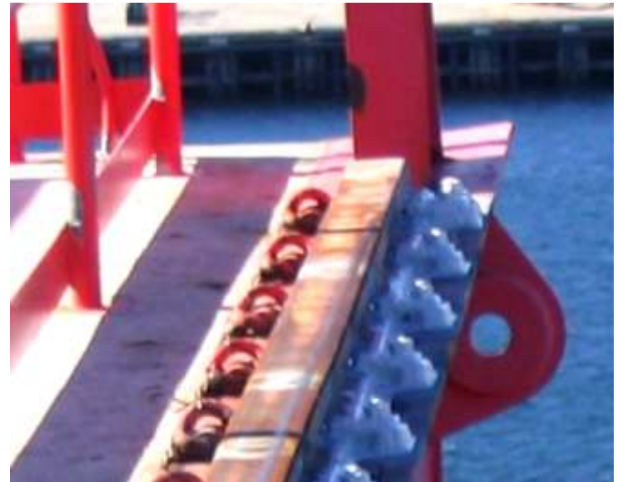
Right: A length of track on the jib showing coated cleats linked with Enviropeel to improve security Below Right: Views of Enviropeel coated cleats
