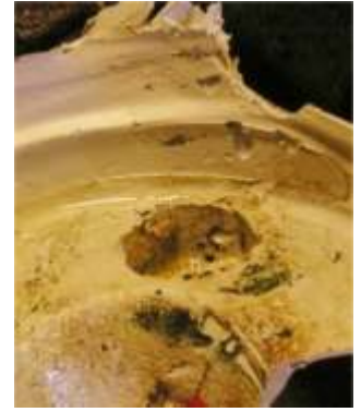
Above: after two years, an application on a flange with severely corroded bolts is cut away for inspection. No further corrosion has taken place and inhibiting oil can be seen on the fastening and in the removed Enviropeel coating.
